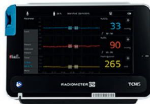
A TCM5 FLEX transcutaneous tcpCO 2 monitor can be added via our optocoupler
